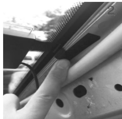
Stick the transparent part of the antenna on the windshield and put the black part on the metal frame.
