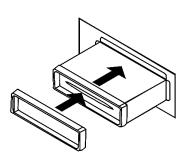
3. Attach wires from the unit to existing wires. See wiring connections diagram. Insert radio into dashboard. Then apply the trim frame to outside of radio.
