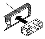
1. After removing the old radio and mounting sleeve, insert supplied mounting sleeve into opening.
