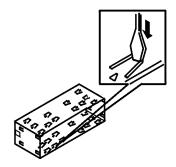
2. Bend the tabs on the mounting sleeve to keep the mounting sleeve firmly in place.
