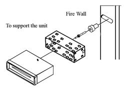
4. Support radio using supplied rear mounting bolt and steel bar. See parts list.
