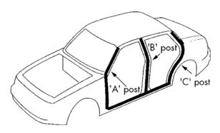
Place the antenna on the windshield near the 'A post'
