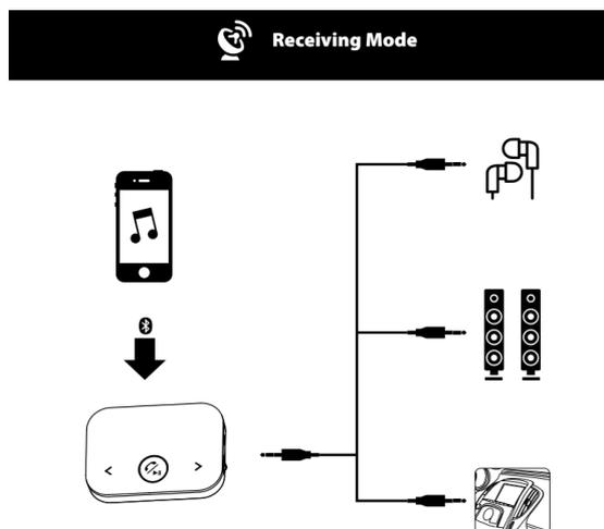
1. When the adapter pair the *Bluetooth* devices, the LED will keep light in blue.
