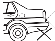
Be sure no other parts of the vehicle falls in the positioning range of the sensors so as to give a false detection.
