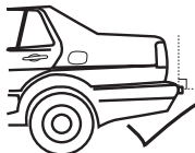
Be sure no other parts of the vehicle falls in the positioning range of the sensors so as to give a false detection.
