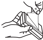
Place the control unit with double-sided tape.
