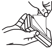
Place the control unit with double-sided tape.
