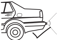
Be sure no other parts of the vehicle falls in the positioning range of the sensors so as to give a false detection.
