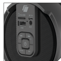
Control panel, USB/SD, AUX-in and charge input 5VDC
