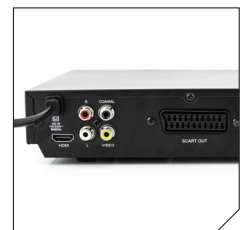
4 ways to connect: HDMI, Scart, composite or coaxial (RCA audio/video)
