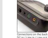
DC-in / Line-in / Line-out / Antenna
