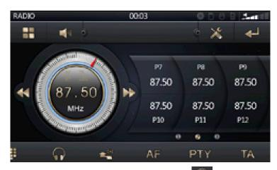
**6. Mono/Stereo Reception Control**In FM radio mode, touch the ST button to select stereo or mono reception.
